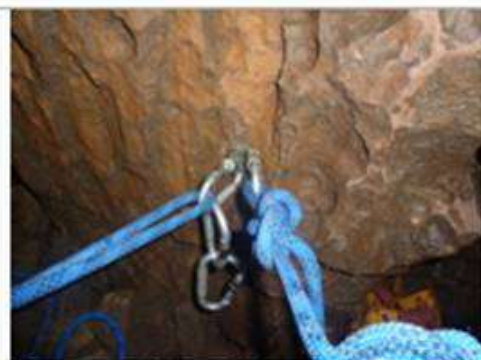
Bottom anchors - 12mm hangers x2 (2 more bolts required)
